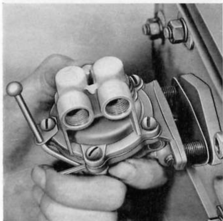
Fig. 45 Fuel Lift Pump
