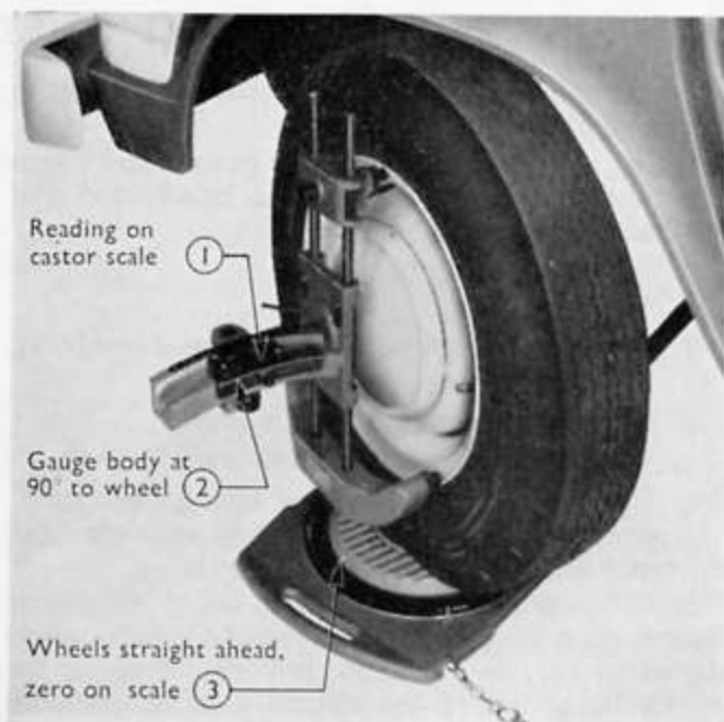
Fig. 16 Castor Angle
