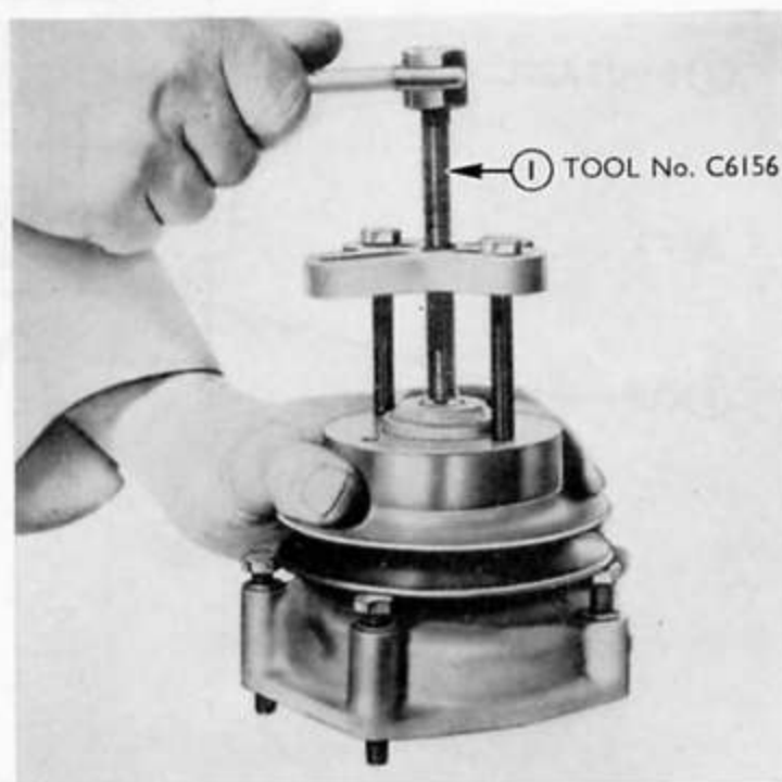
Fig. 7 Removing Water Pump Pulley—Diesel
