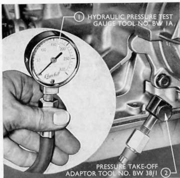
Fig. 70 Checking Line Pressure
