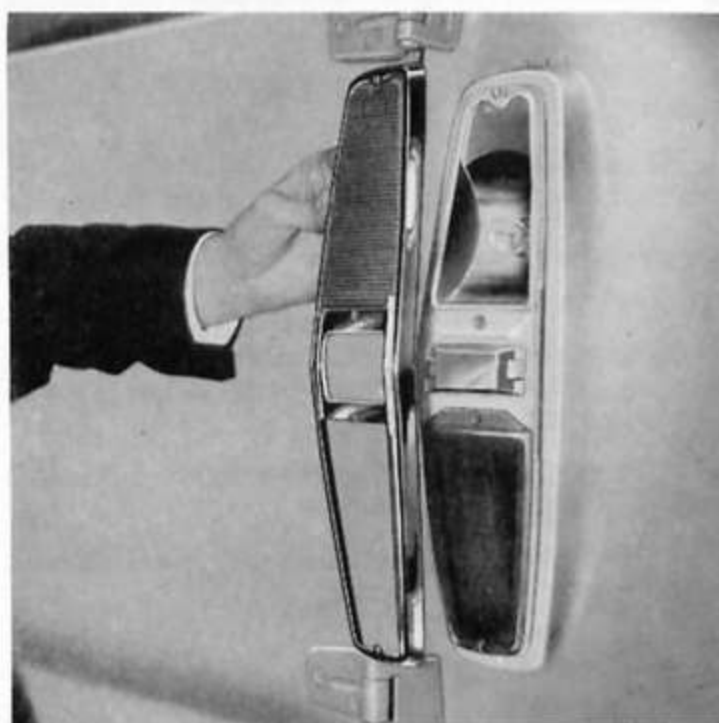
Fig. 4 Replacing a Rear Bulb
