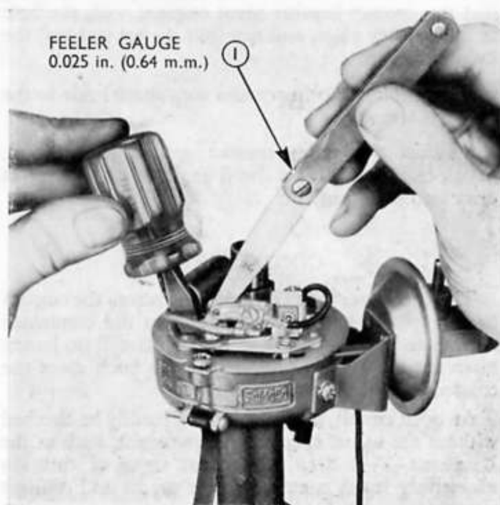
Fig. 33 Adjusting the Contact Breaker Points
