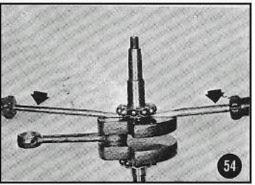
The inner races can be removed from the shaft journal only with a special tool, Pt. No. 09.11.11-26/12. The tool is positioned with the pressure ring in its upper position; then the ring is forced down so that it closes the collet which grips the race in the ball groove. Ensure that only the upper crankshaft web is held during the blows against the ring so that no pressure is exerted upon the crankpin (Fig. 55). Do not clamp in a vise for mounting the puller
