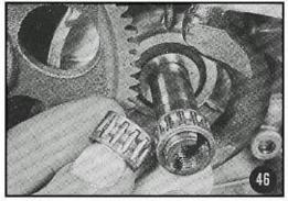
The free crankshaft journal now still holds two needle bearings and a thrust washer (Fig. 46) which must be fitted in exactly the same location with assembly. Worn clutch parts should be renewed rather than repaired.
