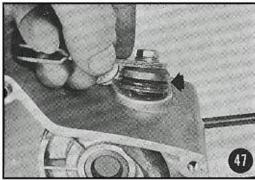
Fig. 47: The clutch control shaft is manually disassembled. The arrow points to the O-ring installed as a seal.
