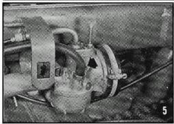
Close fuel valve, if you have not done this before. Pull fuel hose from carburetor simultaneously checking for cracks in the hose (particularly in the area marked by arrow in Fig. 5). Loosen carburetor binding screw (do not remove) (Fig. 6). Pull carburetor off (by turning). The intake manifold may remain screwed to the cylinder; access to the fastening screws is easier with the engine removed.
