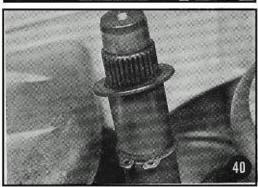
Remove the large gear with free wheeling mechanism; underneath you find a thrust washer (1.0 mm thick) which never needs replacement and supports the gear in the direction of the snap ring (Fig. 40). The snap ring is never removed.
