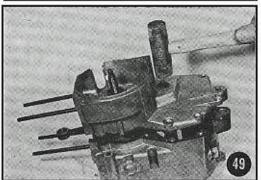
The crankcase halves may be separated without applying force. Just make sure the output shaft does not stick in the bearing, which would cause tilting. Light (very light) blows with a plastic hammer may be helpful (Figs. 49 and 50).
