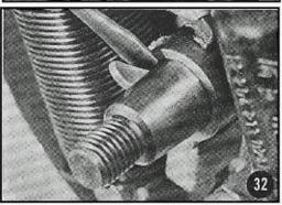
Now unscrew ignition base plate. You may mark its position prior to removal and after having checked firing point and adjusted if necessary. However, it is better to adjust following completion of the repair work (Fig. 34).
