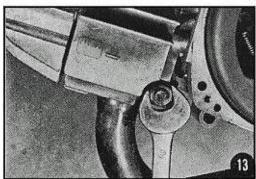
Disconnect exhaust pipe from cylinder (13 mm wrench size, Fig. 13) and unscrew rear muffler mount completely. Caution: Do not lose the flat steel nut piece (Fig. 14). Now, the entire exhaust system may be removed.
