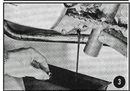
Oil filling capacity 330 cc automatic transmission oil, item No. 215.09.11 K-K 131.
