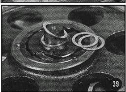
Make sure the washers are not mixed up, because they may be reused for assembly if no shaft or other part must be renewed that influences the length. The exchange of bearings requires no readjustment of the shaft end play since bearings are made to very close tolerances. (Fig. 39 shows the washers on the output shaft; you can also recognize the free wheeling lock).
