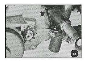
While the upper mounting bolt may be removed without any difficulties (Fig. 21), access to the nut of the lower bolt frequently necessitates the chain guide being loosened and swung upward (Fig. 22).
