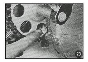
Finally the bolt is pushed through one of the sprocket holes from the left to the right (Fig. 23).
