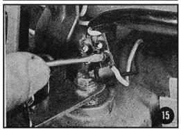
Disconnect the decompression valve cable. The same cable operates also the clutch for flying start, i. e. when the engine is stopped and is to be started by the motion of the vehicle. Cable setting must not be changed! Disconnect from clutch lever on transmission casing (Fig. 16).
