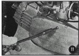
The plastic cover on the left engine side over the flywheel magneto may be unscrewed (Fig. 11).
