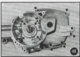
The two crankcase halves are held together by nine screws. The four screws inside the magneto housing are M 6 x 45 with fillister head; the remaining five are oval head countersunk screws M 6 x 30 (Fig. 48).
