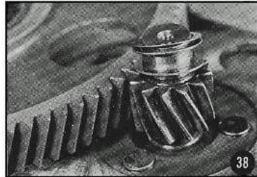
Watch the compensating washers located on the crankshaft journal as well as on the output shaft (Fig. 38 = crankshaft with clutch housing).
