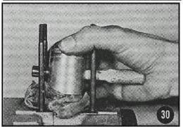
Use a hardwood drift for forcing the gudgeon pin out of the cold piston. If excessive force has to be applied, please check the lock ring groove for burrs which may have built up there (Fig. 30).
