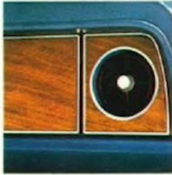
Aeroflow ventilatic systeem.
